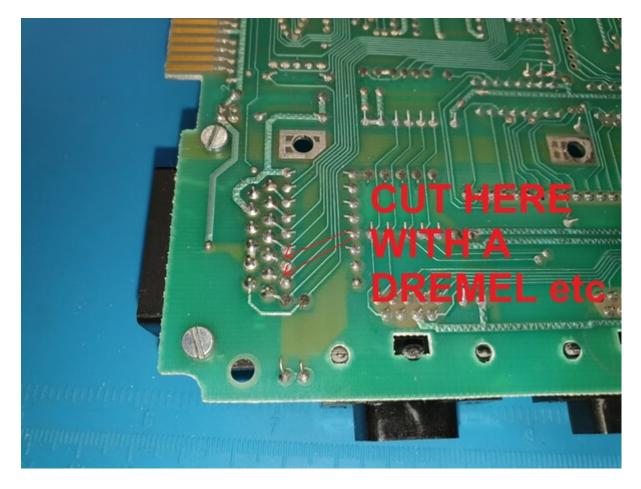
Use a dremel or similar tool and cut the traces between SIO jack pin 3 and 5 and their capacitors.
